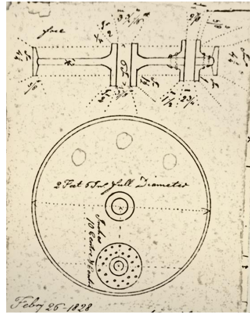
Figure 1 Sketch made by Timothy Hackworth in his notebook dated 26 th February 1828 of the plug wheel (NRM HACK 1/3/2/1).
