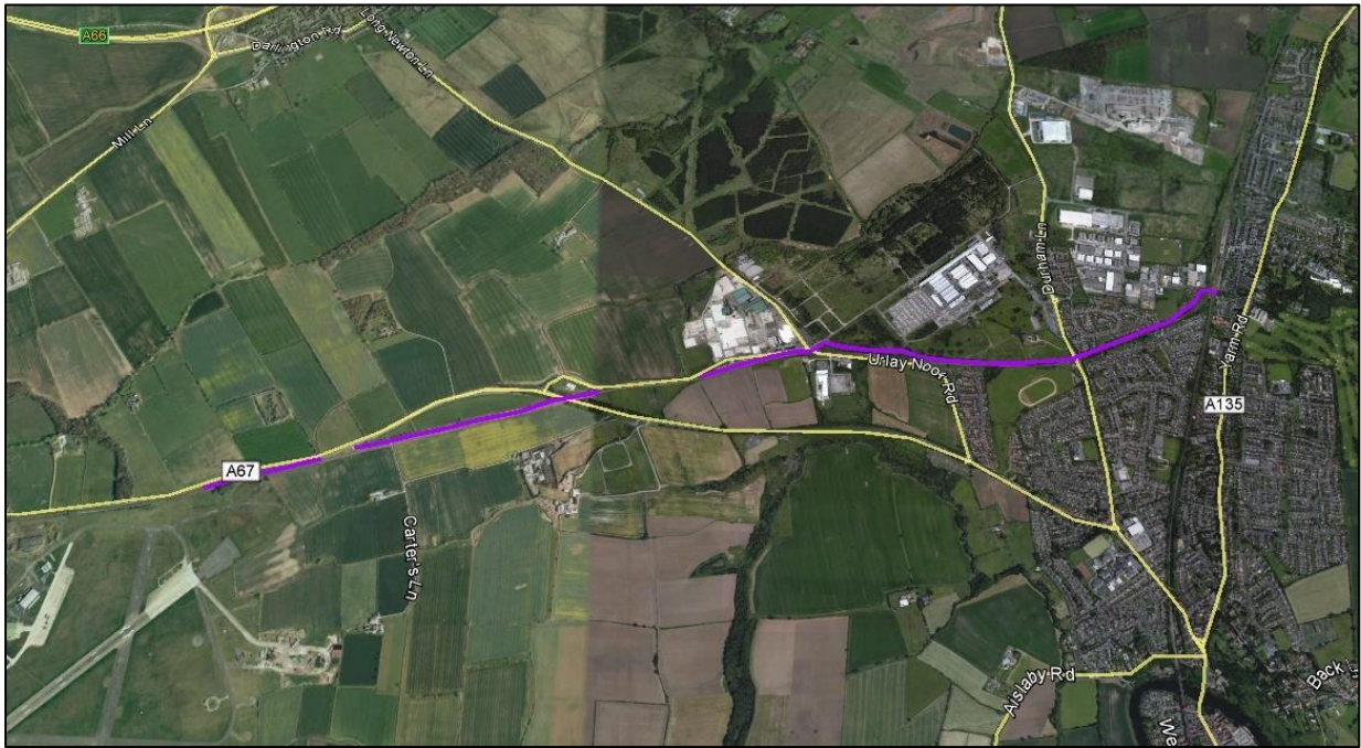
Figure 7. A cycle path or footpath could be established in places using disused roads (Carter's Lane), existing paths associated with industrial complexes (Durham Lane), disused sidings north of Allens West, waste ground and areas where there are wide verges (shown in purple). Other stretches have reasonable verge sizes too so it may be possible to carve out a new path without resorting to acquiring new land.
