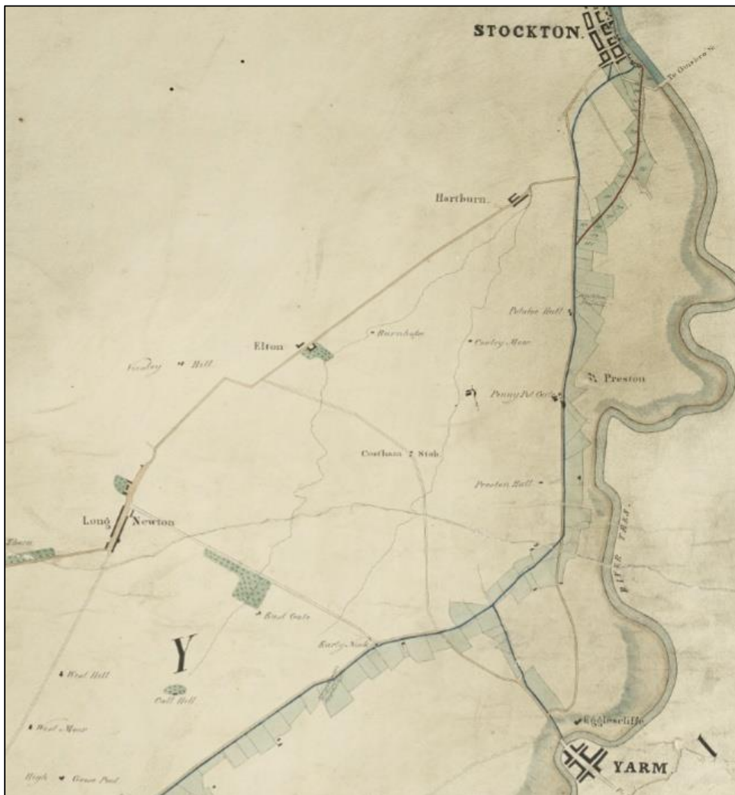
Figure 2. George Stephenson's map of the proposed S&DR railway, showing his proposed altered route into Stockton surveyed in 1822 (DRO Q/D/P/8/1). The blue line marks the route, as originally conceived by George Overton. Overton's route was uncontroversial as it followed a gentle decline into Stockton with no major engineering issues to overcome.
