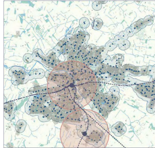
Figure 5. Transport Accessibility: Parts of the design code may allow an increase in densities or building heights in areas of high public transport accessibility. If this is the case, it will be important to have a plan showing public transport accessibility such as a public transport accessibility level plan or equivalent.
