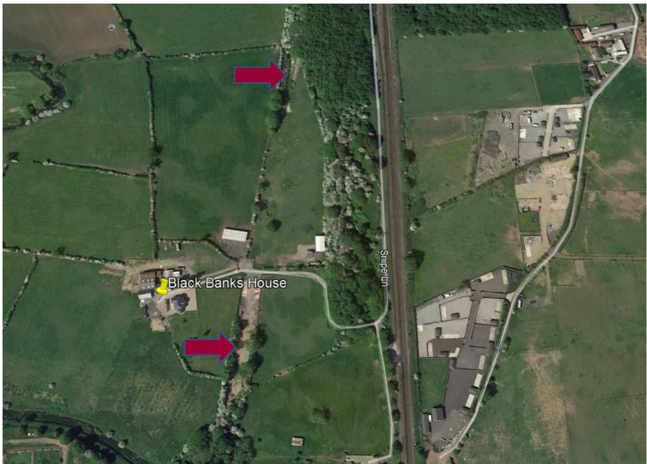
Figure 54. Areas of current extraction of trackbed earthworks at Black Banks (marked with arrows)
