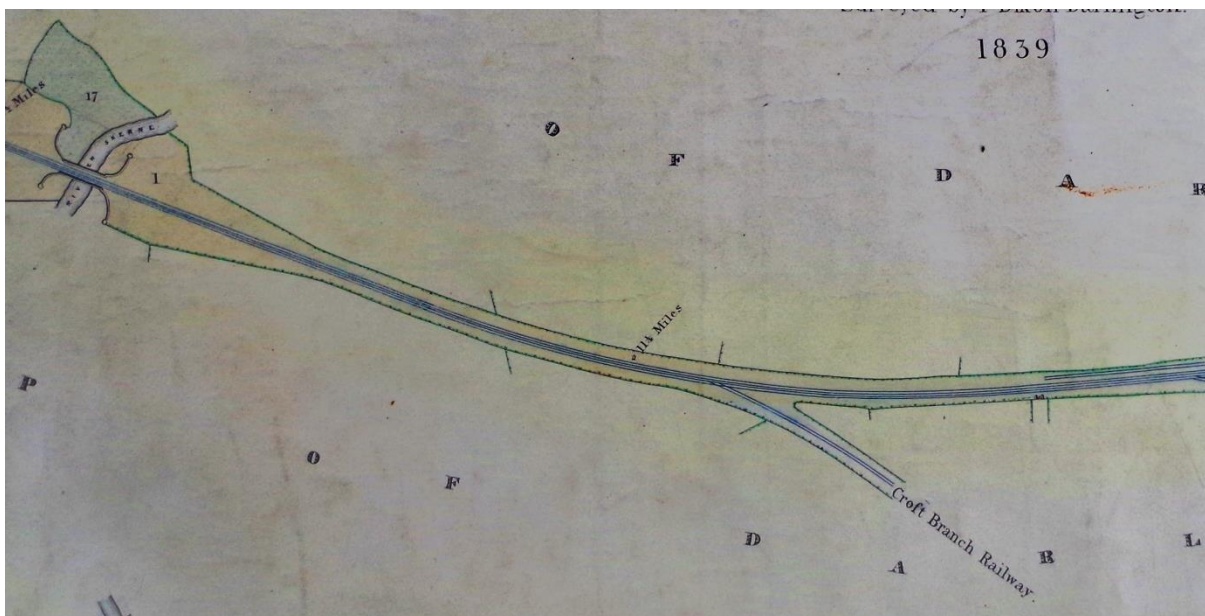
Figure 6. The start of branch line as constructed and surveyed on Thomas Dixon's plans of S&DR property in 1839. The bridge on the left with curved wing walls and circular end piers is the Skerne Bridge in Darlington (RAIL 1037/456)
