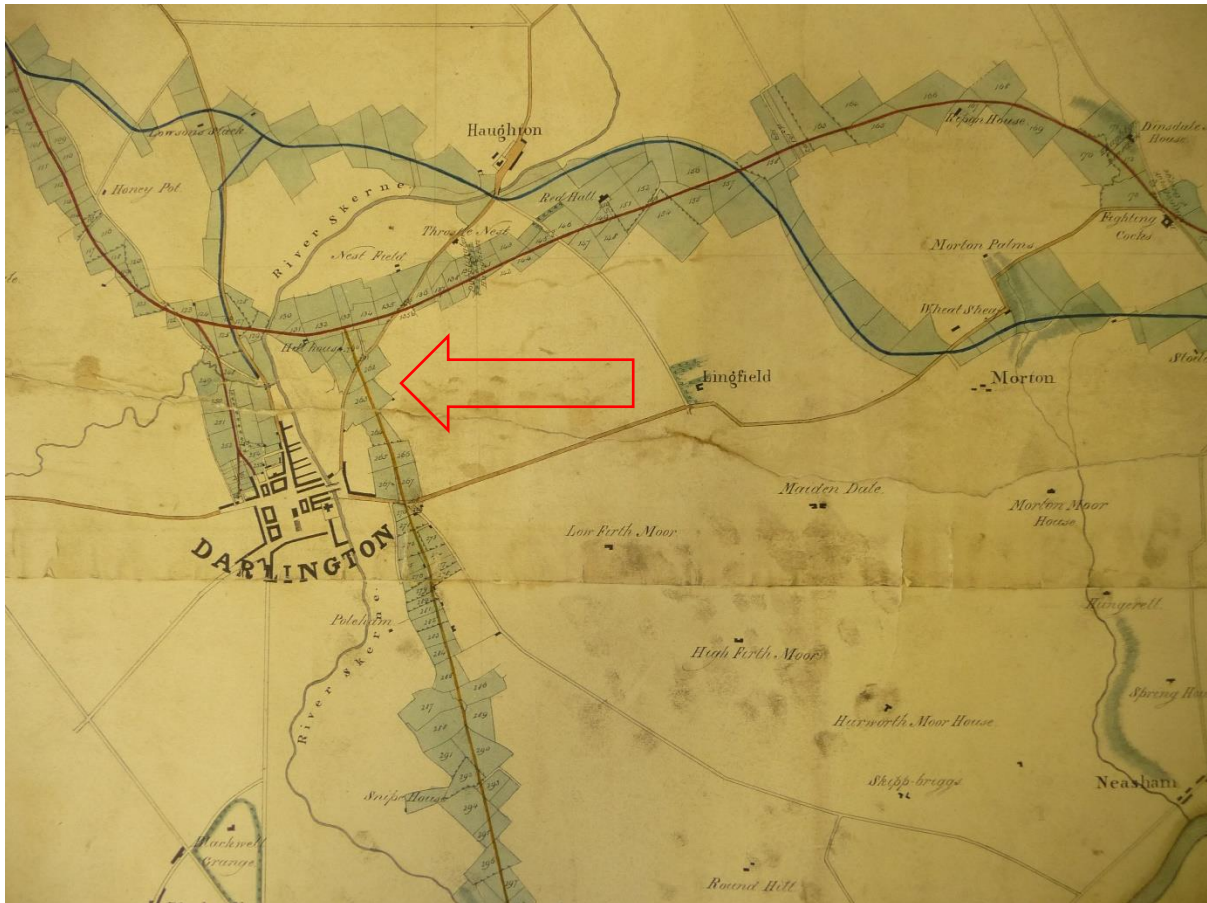
Figure 2. George Stephenson's proposed route of the Croft branch line with an improbably sharp right turn leading from the main line at Hill Top House (DRO Q/D/P/8)
